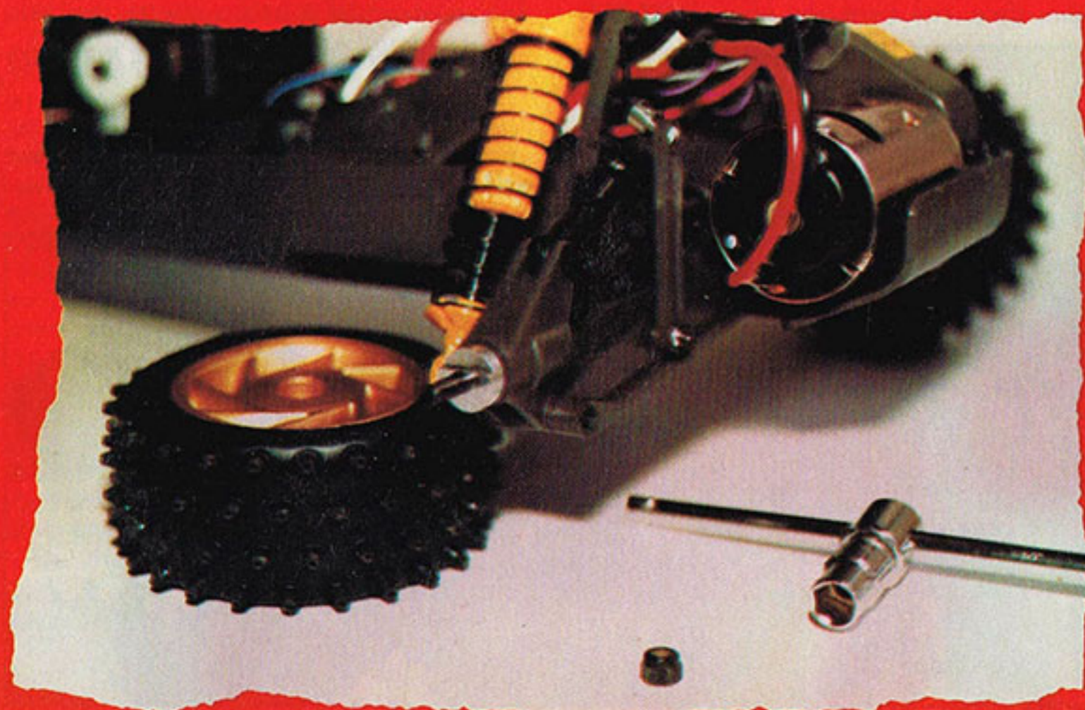
Below, rear of car with wheel removed to show slot drive to hub.
