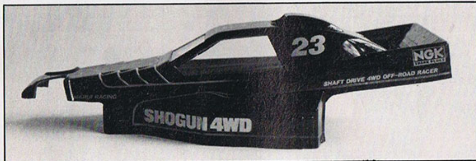
Body shell, note the strengthening moulding around the front shock absorber cut-outs.
