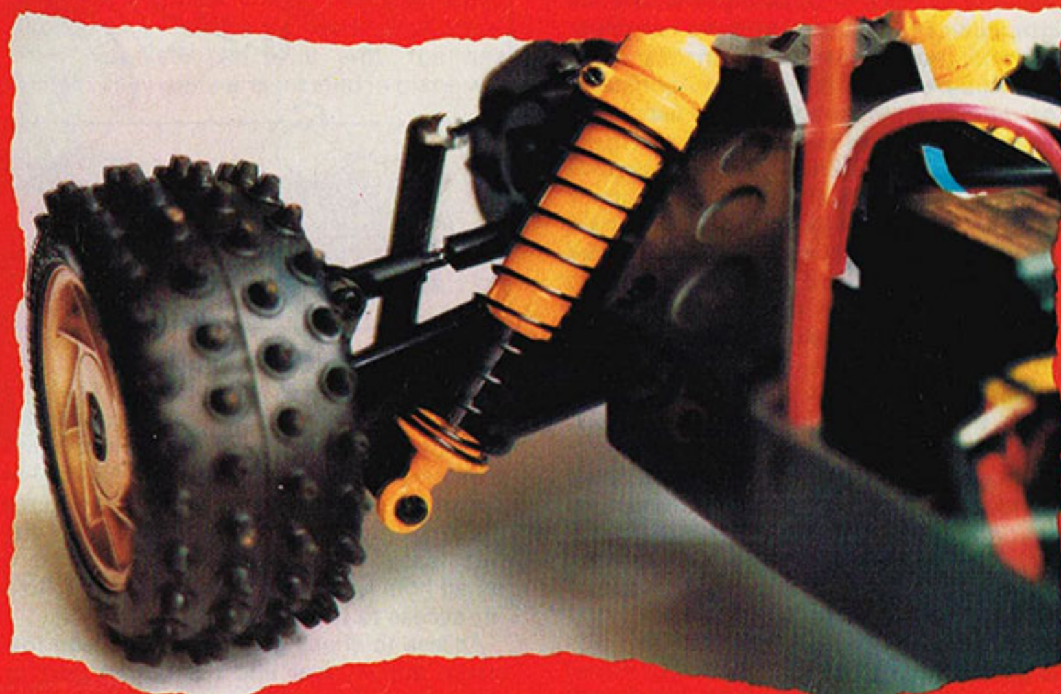
Above, long travel rear dampers very smooth plastic chassis see reflection of damper. High grip tyres.
